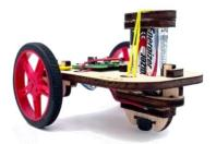
Within the Horizon Europe OpenSwarm project (www.openswarm.eu, 2023-2026), we are developing the DotBot (www.dotbots.org), an open-source robotic platform which features a printed circuit board and two motors installed on a lasercut wooden chassis, with a lighthouse receiver for mm-accurate localization. As an open-source platform, DotBot is being designed for education and research. We are working on educational and research kits; we target students at the primary school, high school
